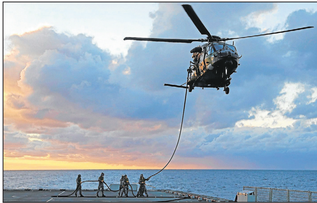
HMAS Choules' embarked MRH-90 aircraft, Posiedon-14, conducting helicopter in-flight refuelling training operations, during a sortie, off the flight deck off the coast of South Queensland.
