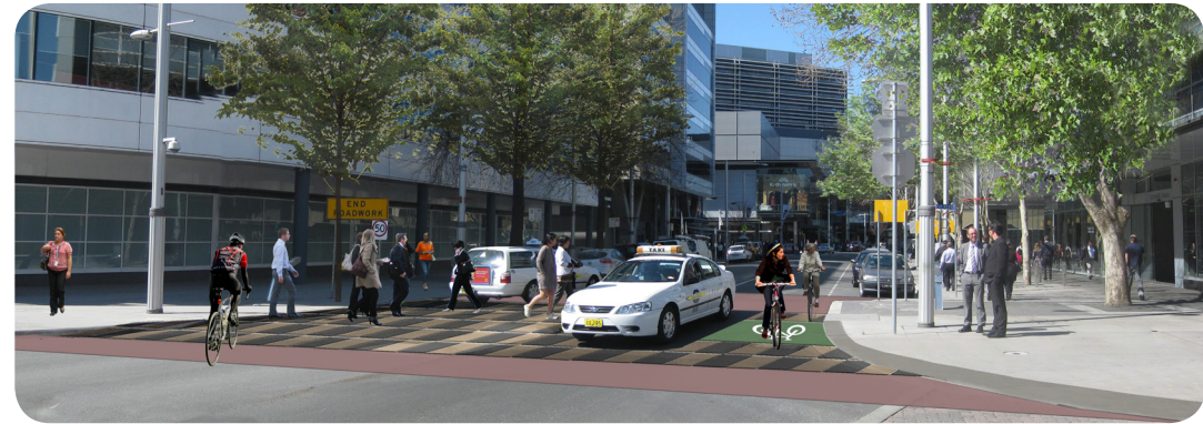
MORT STREET/ BUNDA STREET RAISED THRESHOLD WITH DIFFERENT PAVING
